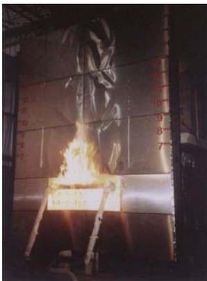
Example of fire test for roof
