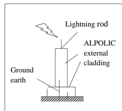
considerable damage will not occur in most of the ALPOLIC panels in the building. But the impact of the lightning is so intense that the struck panel itself will be completely damaged.
