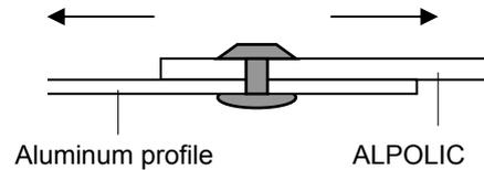
In actual installation work, the position of joining hole is important. When the hole is positioned in the proximity of panel edge, its strength will be lessened and may be unsatisfactory. Normally, the distance from hole-center to panel edge ( $e$ ) should be larger than twice the hole-diameter ( $D$ ). Namely,  $e > 2 \times D$ . Refer to “Appendix 6: Strength of joining hole” in Section 4.
