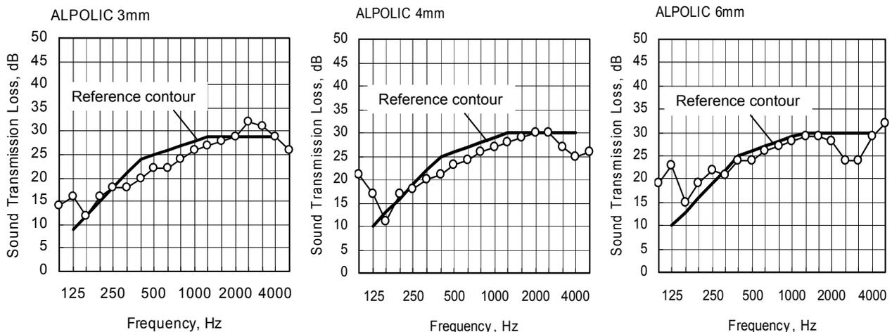
**Fig. 2-1 Sound transmission loss**
