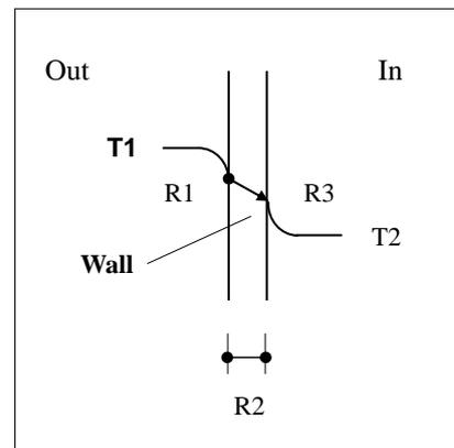
In the same manner, we can calculate the heat transmission of actual wall systems. Table 2-11 is a calculated example. The calculated value is called the heat transmission coefficient, U-value ( $W/m^2 \cdot K$ ) or K-value ( $kcal/m^2 h \cdot ^\circ C$ ). A lower U-value means less heat flow or higher heat resistance. As we can see in the table, covering the wall with ALPOLIC cladding improves the thermal insulation effect by
